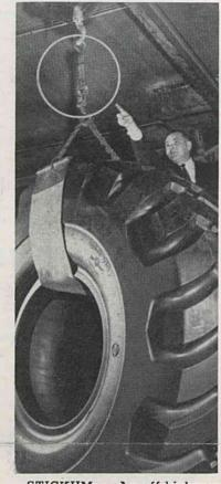
STICKUM - An off-highway tire weighing nearly 2,000 pounds is here suspended by two square inches of a newly-developed Loxite adhesive produced by Firestone. Richard Garling, senior chemist who helped develop the metal-to-metal adhesive, points to a carbon-steel strip (encircled) overlapped and held together by the Loxite. The high-strength adhesive will be used in the automotive industry. It has been pull-tested as high as 2,500 pounds per square inch and can be applied even to oily metal.
