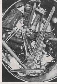
DOWN IN THE BARREL Defective tools are a rarity these days. But wrenches aren't hammers, handles aren't crowbars, hacksaws aren't wedges and pliers. Using right tool for right job is the answer to much of this kind of waste problem.
