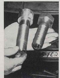
Here are two bolts with identical threads and diameters. The one on the left costs \$15.70 and the other, \$1.47. Which one would you use for an ordinary job?
