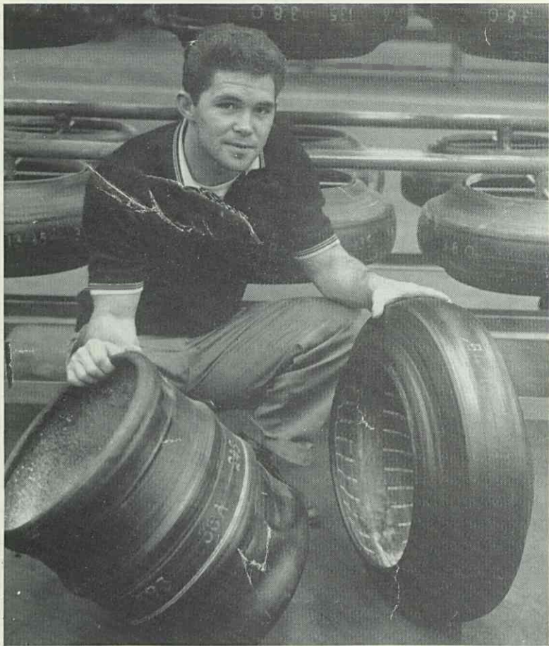
A FIRESTONE TIRE BUILDER compares an uncured conventional passenger tire (left) in the familiar barrel shape, with an uncured radial-ply passenger tire (right). At this stage, both tires are ready to be placed in curing molds. Longer tread life, quicker steering response and better cornering are features of tires built with radial plies.
