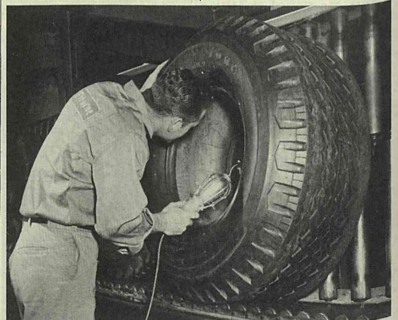
DUPLEX tires, new single tires to replace duals on tractor-trailer rigs, were introduced in 1960 and 1961.
