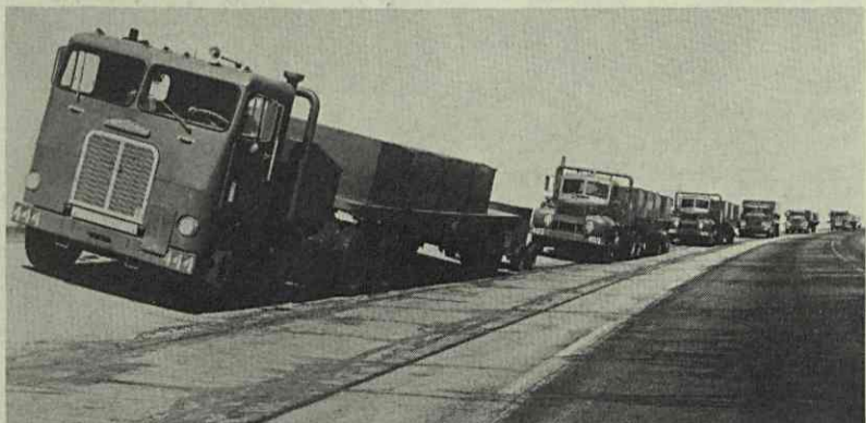
AT PEAK PERIODS of tire testing, this fleet of trucks circles the Firestone Test Center track at Ft. Stockton, Texas, 24 hours a day. The 7.7-mile track, capable of safe operation at speeds up to 130 miles per hour, provides an excellent site for tractors and trailers running at highway speeds with normal loads or heavy overloads.
