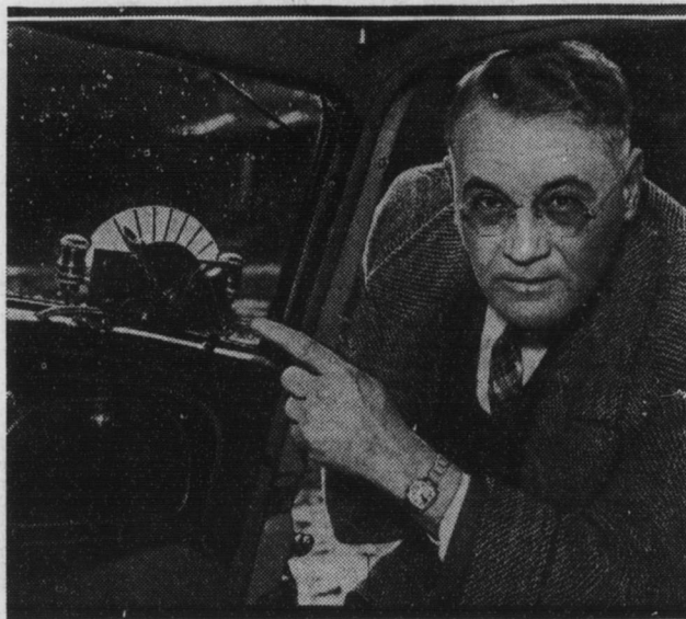
J. J. Huescher of Minnesota is shown with his regulating rheostat mounted on the cowling of a car just inside the windshield. The position of the dial determines the maximum speed of the car. A white light on the left burns at proper speeds, and a red light at right burns when the speed is excessive.
