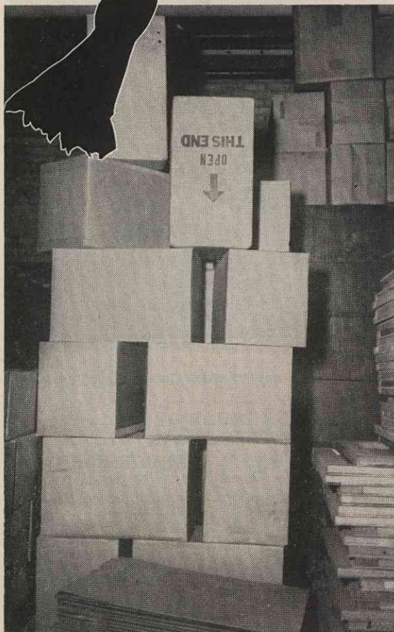
The stacking of cartons should always be done with CARE, and NOT as shown above. In fact, any material that is not stacked properly can create a hazard and contribute to serious injuries.
