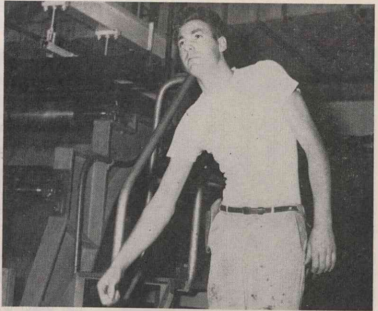
Jim Fisher, casting operator, by raising his arm to a front horizontal position, tells fellow operator to change to rod so that the width of the cellophane sheet may increase to the proper size.
