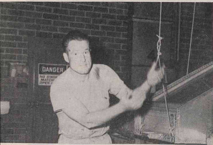
This lifting motion, carried out by Cecil Smith, a casting operator, signals for the removing of the hopper from the wet-end of one of the casting machines. Viscose is forced through a narrow slit in the hopper and coagulated by an acid bath, transforming a viscous liquid into a thin film.
