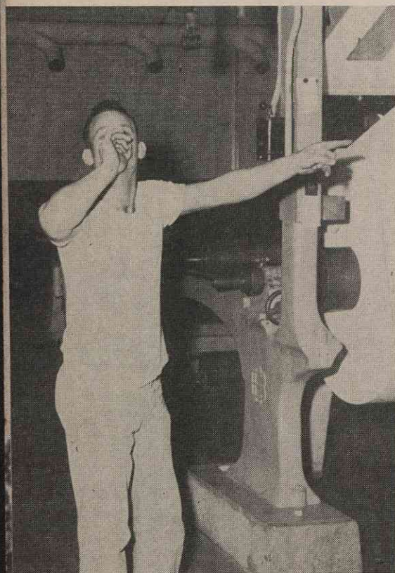
With this signal Charles Tinsley, a Third Hand, tells the machine tender that blow-wrinkles have begun appearing in the paper.
