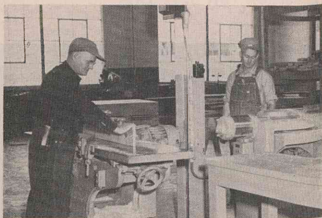
Left: Thurman King and Carl Baynard stack pallets, made in the Carpenter Shop, which will be used by the shipping department. Above: Joseph ("Uncle Joe") Kornowski uses the jointer while Clarence ("Swivel") Allison runs a short length of board through the planer.
