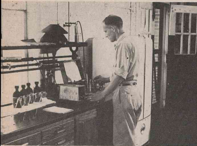
To determine silica content of boiler water, tests have to be made regularly. William Kuykendall is shown making a test in the laboratory.
