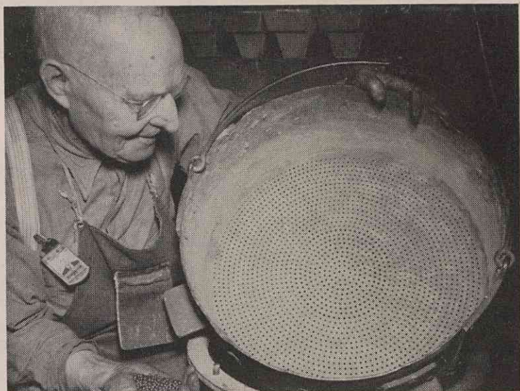
A dropping pan for No. 6 shot, containing 2,400 holes through which molten lead pours and is separated into droplets.
