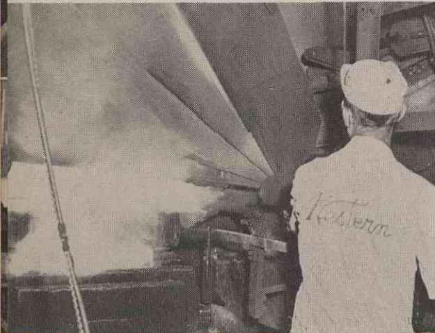
Pouring molten brass into a mold in The Cast Shop is a delicate operation. Here the furnace operator is shown carefully watching over a typical pouring. The furnace is hydraulically tilted until the last bit of brass has been poured into the mold. Critical supervision of pouring is necessary in order to cast a high quality bar.
