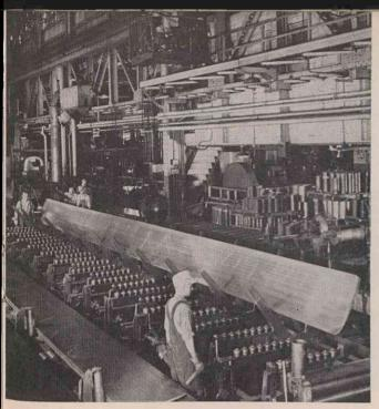
After leaving Hot Mill, brass bar goes first to straightener roll, visible at extreme right. Bar then proceeds to milling machine which cuts off scale from original casting operation and removes any defects present. Above, milled bar is being flipped over to the rack of bars at the left.
