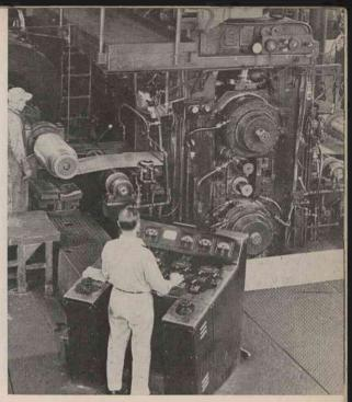
Brass is rolled to very fine tolerances by experienced operators at the East Alton mill. After repeated rollings on various mills, a coil of brass might be stretched out to a length of more than five thousand feet and perhaps nearly as thin as a leaflet of Ecusta cigarette paper.
