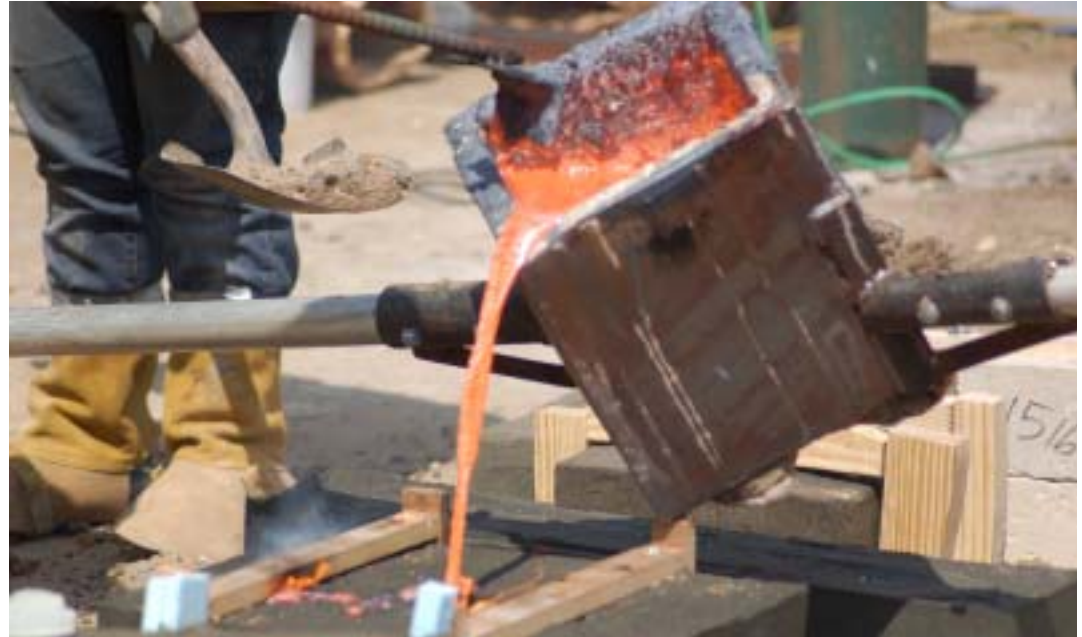
Molten iron is poured into a sand mold
