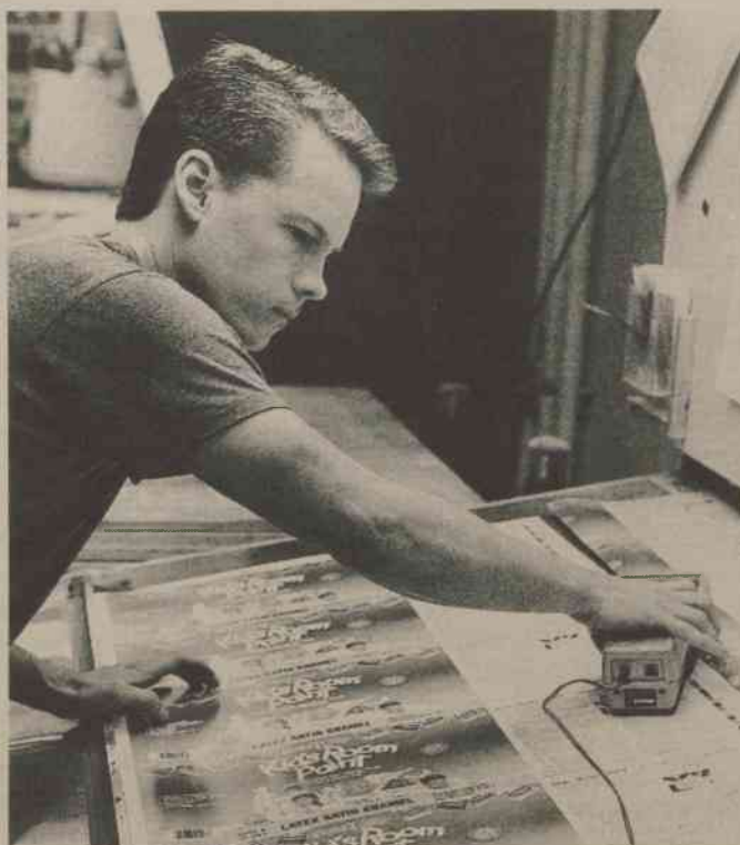
Todd Scruggs ('85), left, is a head pressman with the graphic arts division of Sherwin-Williams Co., of Greenville. Scruggs, who operates a 6-unit, 40-inch Kormori offset press, is shown taking electronic readings of the color reproduction work.
