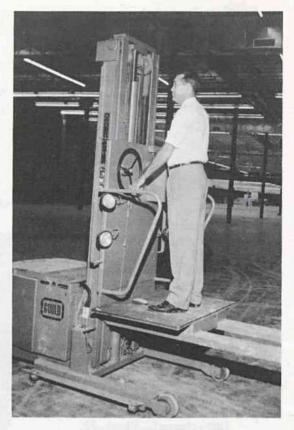
E. C. Tatum, Jr., superintendent of the finishing plant in Kernersville, becomes acquainted with the ORDER-MASTER lift to be used in the stock room of the new plant. The lifts will be used in the rack sections which are 15 to 20 feet high. An order clerk will be able to operate the truck from any height.
