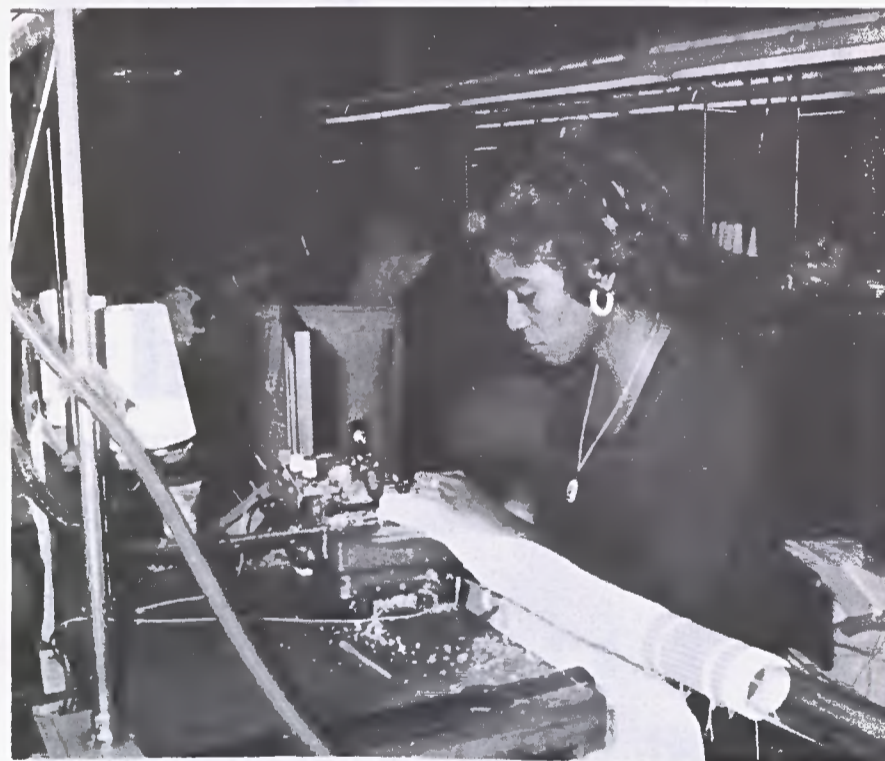
Christine Stone seams the toe of a tube sock on an Union Special Seaming machine. The sock is around a clear tube which uses suction to turn the sock wrong-side-out so that she can seam the inside of the toe, and when the seaming is finished, the tube carries the sock to the collection bin.
