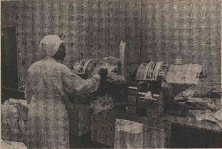
LABELLING —Laundry worker Mary Stevens labels all soiled laundry which is brought to the building for processing. Prior to labelling, soiled linen is separated and classified into flat work (sheets) or dry work (bath towels, patient gowns, etc.) and weighed. It is then placed in chutes destined for the washing machines.
