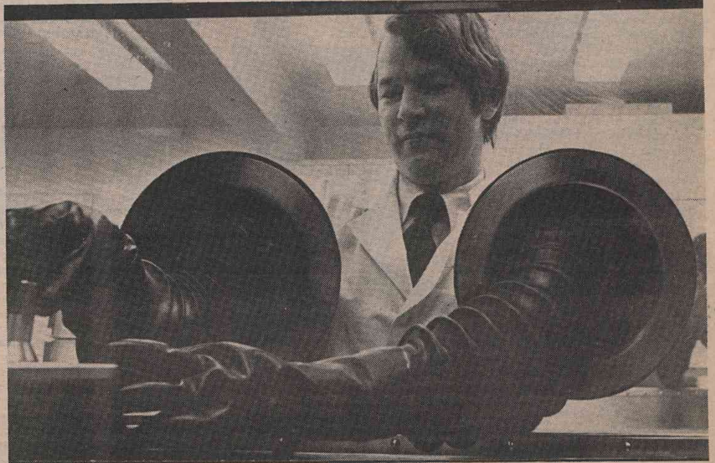
WHAT A VIRUS SEES AT DUKE—This is a "virus-eye view" from the inside of a containment line device, designed to protect scientists while they study viruses at the recently opened Animal Laboratory and Isolation Facility (ALIF). Dr. Darell Bigner, associate professor of pathology and chairman of the ALIF committee, demonstrates how the accordion-like protective rubber gloves work. (Photo by Jim Wallace)
