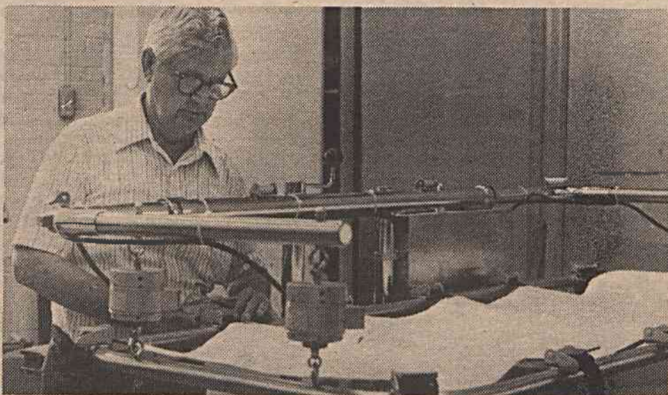
HELP FOR PATIENTS —Billy Barber (above), manager of the Surgical Instruments Shop, adjusts the straps to attach a mat to a portable weighing unit built for thoracic surgery. (The mat would remain on the patient's bed.) Raising the frame so that it lifts the patient slightly off the bed gives a highly accurate reading. On right, Barber points out some equipment in the shop to its founder Dr. J. Deryl Hart, first chairman of the Department of Surgery and president emeritus of the university. The adjustable stand in the foreground holds a hammock-type bed for an infant in the Intensive Care Nursery.
