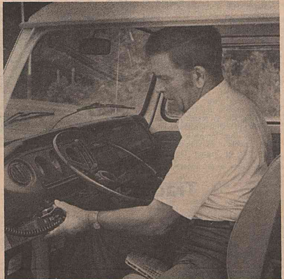
THAT'S A BIG TEN-FOUR—CBers can prevent theft of their radios by following the example of F. A. Ward, parking attendant, and installing a quick-release mounting. A simple pull of the lever and it slides right out to be locked in the trunk or carried inside with you. For a related story and photos see page 3. (Photo by John Becton)
