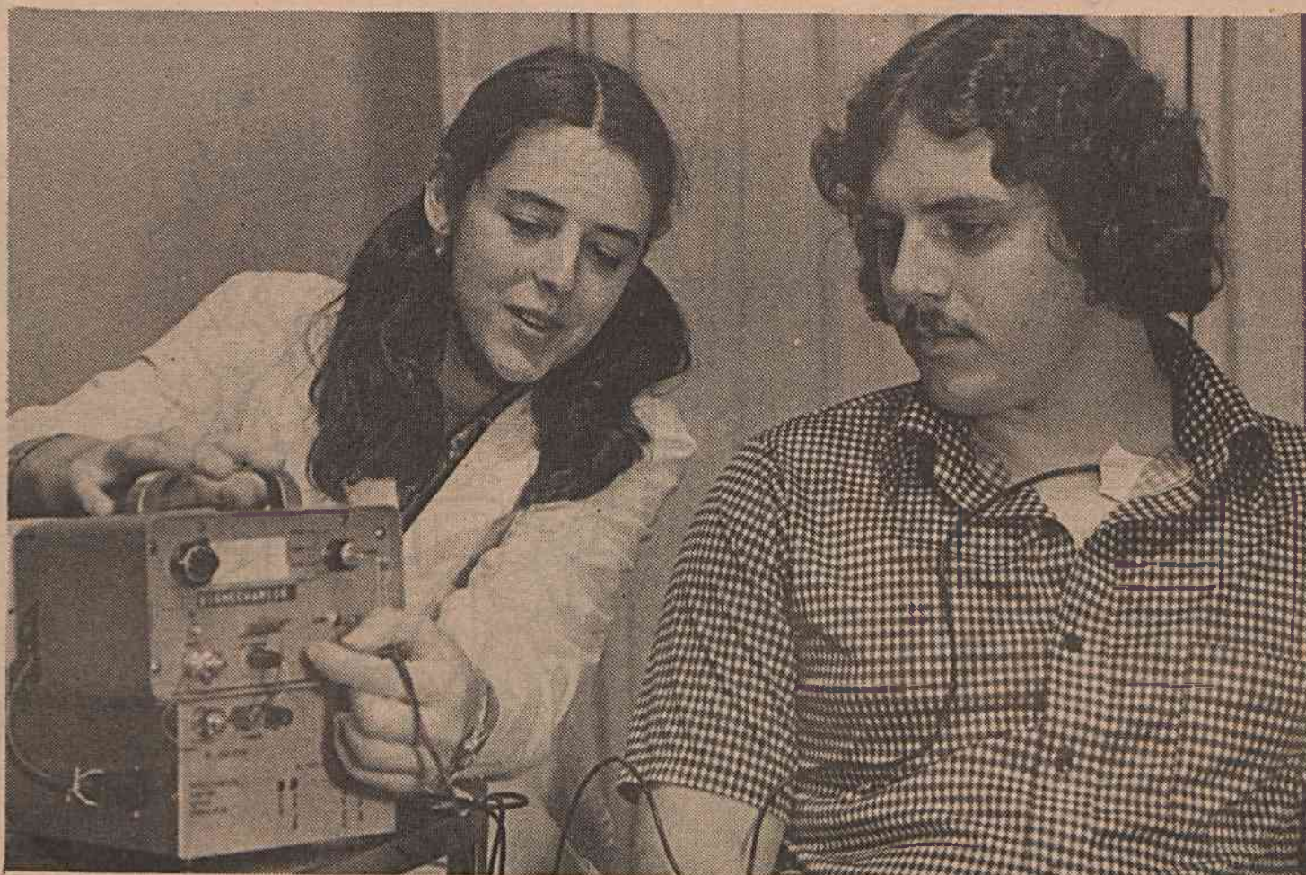
GETTING ADJUSTED —Duke University Engineering student Carolyn Cohen demonstrates how a respiratory pacemaker she designed and constructed will be attached to paralyzed patients to help them breathe more easily in the hospital. The device, already proven effective in
