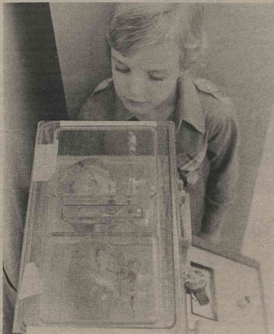
IT'S THE REAL THING —Eight-year-old Marc Hawley gets a close look at a pair of kidneys that were hooked up to a Waters Transport Module, a portable kidney transport machine which keeps the kidneys viable when they are being moved to a transplant site. The machine supplies the kidneys with necessary gases (O 2 and CO 2 ) and maintains a constant 7°C temperature to retard cell breakdown. Marc is the son of Carol Hawley, former secretary to Dr. James F. Glenn, professor and chief of the Division of Urologic Surgery. (Photo by Parker Herring)
