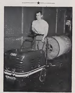
THE EASY WAY:—Hauling beams at the Blanket Mill has been made easy by use of the Clarkette No. 5 towing tractor shown above. The gasoline powered tractor is used for hauling beams from the storage area near the warpers to the slashers in the weave room.
