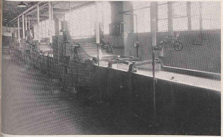
he order has been placed for a latest-model Sargents 4-bowl continuous skein scouring machine for the arastan Mill. The new unit will give improved quality of scouring and the extra capacity needed for two idditional Clark needle looms now on order. Building alterations are under way and will be completed the time the new unit is shipped in mid-August. Picture shows type of machine being purchased.
