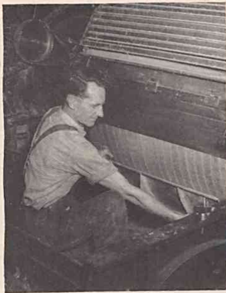
CARD OVERHAULER , Clyde Donaldson and his helpers are completely rebuilding all Towel Mill cards.
