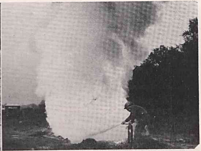
BURNING OIL AND GASOLINE is quickly brought under control by Duncan West in another demonstration showing greater knock-down power of modern pressurized dry powder fire extinguisher.
