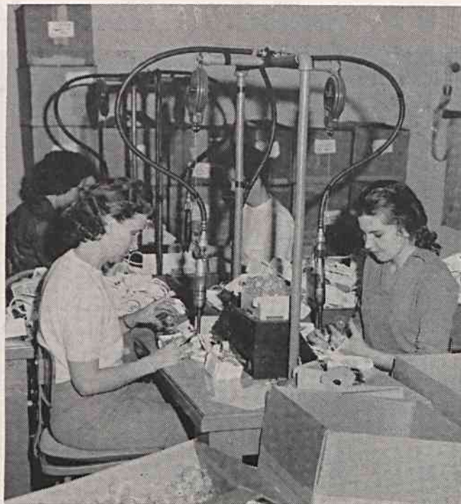
Pat Gambill and Leora Evans (in foreground) attach dials to control cases. Cases also are molded at the plant.
