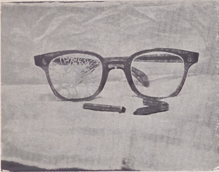
Cracked lens in his safety glasses shows what would have happened to Gary Grogg's eye if he had not been protected.
