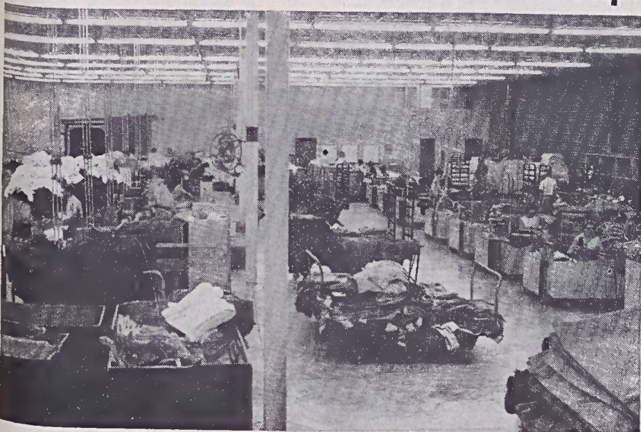
This over-all view shows the enlarged Drapery Department at the Bedspread Finishing Mill. The machines to the left are for pleating and sewing on rings; the hemming operation is performed by the machines at the right.
