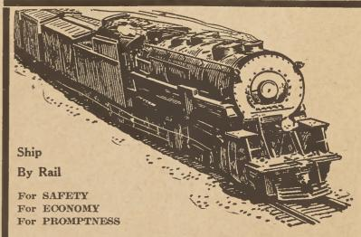
The railways have reduced the number of locomotives in use by increasing the power of the average locomotive. From 1916 to 1938 the tractive power of the average steam locomotive has been raised from 33,188 pounds to 49,803 pounds, an increase of 50 per cent.
