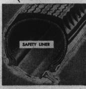
Here is a tire with new principles of design and construction which protects you against dangerous blowouts. In this new safety tire, the tube is replaced by an air-tight butyl Safety Liner that's bonded to the inside of the tire. No tube to pinch, tear or suddenly explode when injury to the tire body occurs. Air loss is so gradual there is ample time for safe,
