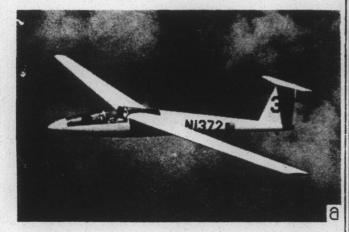
SLEEK, NEW SAILPLANE, designed for do-it-yourself builder, is capable of reaching speeds of 150 miles an hour. The craft is available only in kit form. Completion requires only hand tools, rivet gun and air compressor. The plane has a wingspan of 54.6 feet and is nearly 24 feet long. The aluminum surface will not warp from temperature and humidity changes.
