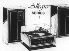
Model H584W • Features Allegro Series I Amplifier with 2.5 watts min. RMS per channel from 100 Hz to 10 kHz into 8 ohms at no more than 1% total harmonic distortion. AM/FM/Stereo FM Tuner. Stereo Precision Record Changer. Shown with Zenith Allegro 1000 speaker systems. Simulated wood cabinet; grained Walnut finish.
