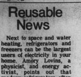
home. Amory Lovins, a physicist, and energy ac-tivist, points out that modern refrigerators often function like heaters as well as coolers. He explains that old time refrigerators used to have the motors on top so that the heat they gave off would rise above the refrigerator. Today's appliances feature the motor underneath the refrigeration compartments where heat from the motor helps heat the food, causing it to run more often.
