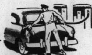
THE OLD WAY—Gas filler cap on fender... unhandy to reach from far side... unsightly.
