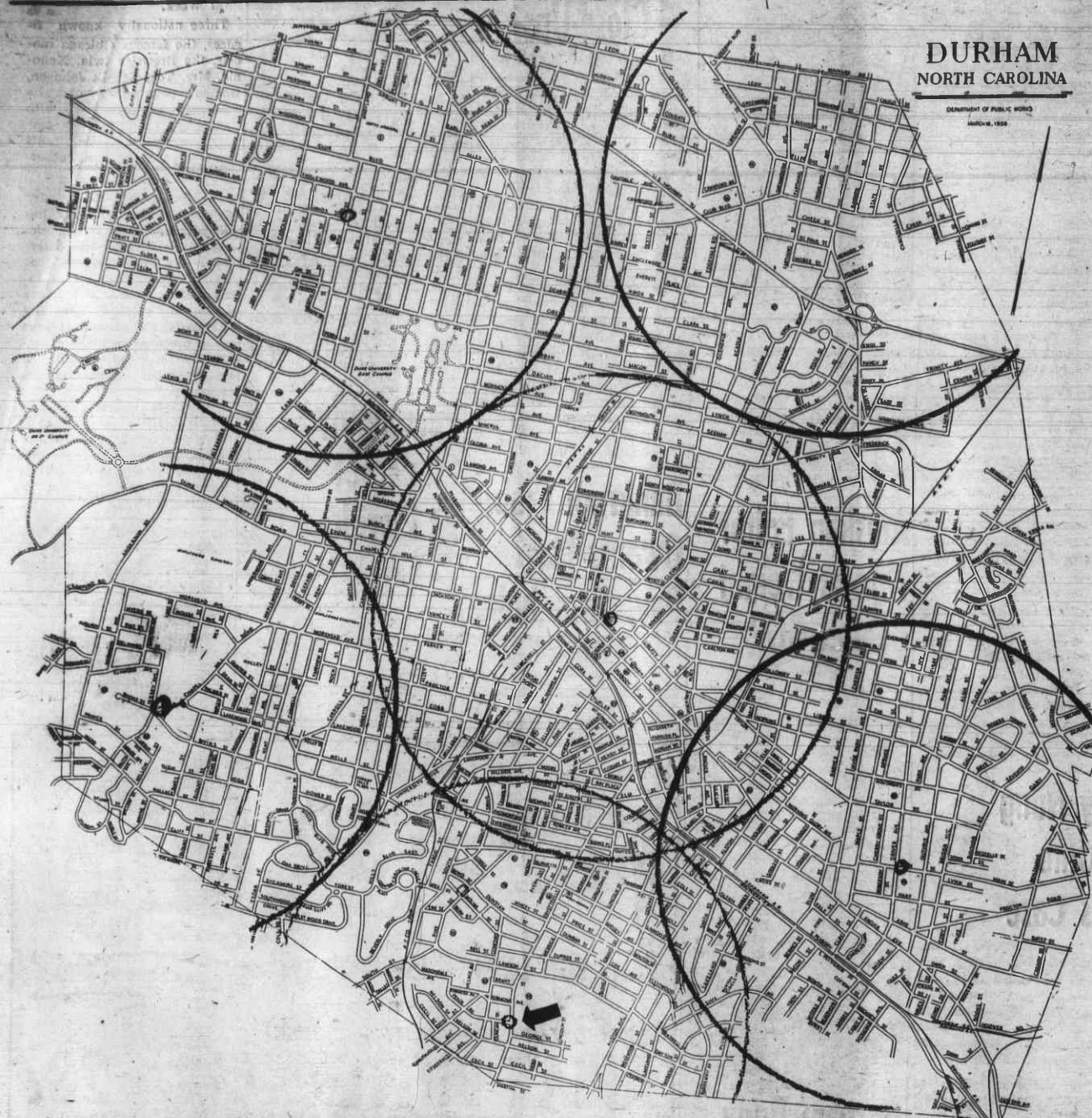
Arcs inscribed on the above map of the city of Durham show the location and area served by the existing fire stations in city. Proponents for the location of a fire station in Haiti section at the intersection of Pekoe and Fayetteville Streets point out that the map indicates this site would afford the city maximum coverage with a minimum of overlapping.
