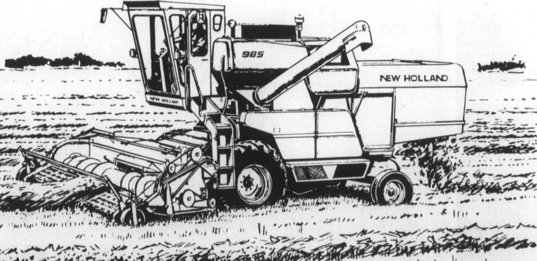
MODERN COMBINES can be fitted with a variety of attachments for harvesting different crops. This combine, a New Holland model 985, is equipped with a windrow pick-up header for grain crops that were previously cut and windrowed. Other headers cut crops directly and feed them into the combine.
