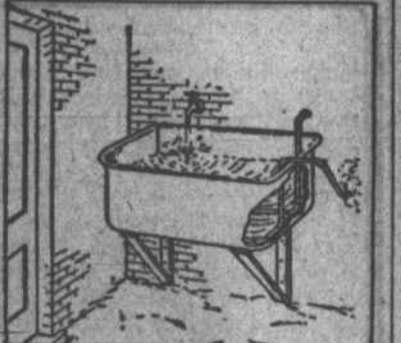
Using Exhaust From Gas Engine to Keep Water in Trough From Freezing.
