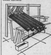
A section of old inner tube about two feet long is slipped over the peeled surface and bound in place. The post is then laid on a rack with the large end about two feet or more higher than the small end. In a short time the preservative, con-tained in the tube, will begin to flow into the sapwood of the post, forcing the natural sap out at the small end. When all the preservative has flowed from the tire tube into the wood, the tube is removed and the post taken from the rack.
