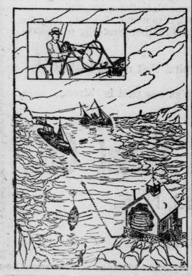
large area around the vessel. Pumped from a tank on deck, the fluid passes far out from the boat to umbrellalike devices of canvas that are set floating in the sea. It can be used for large or small craft, or from lifeboats while making their way through heavy waves in the event of
