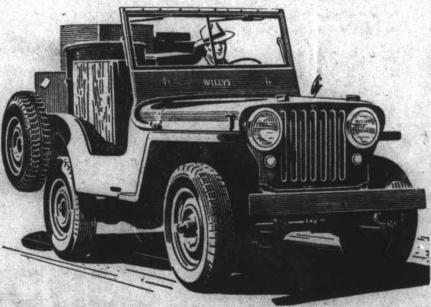
THE UNIVERSAL "JEEP" works as a pick-up truck for loads to 1,200 lbs., using 2-wheel drive for highway economy, 4-wheel drive to get through mud, snow and sand or travel cross-country.
