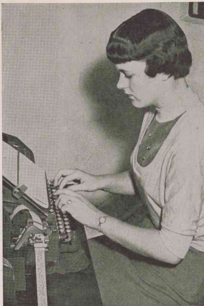
A NEW OCCUPATION FOR WOMEN—Pretty Jean Sykes of Conway, is shown operating the keyboard of a Teletypesetter perforator, the machine that has opened up an entirely new occupation for women in the newspaper field. The tape from this machine (shown in the lower left hand of the picture) is fed through an apparatus attached to a typesetting machine and automatically sets type for newspapers. Miss Sykes is a student at the Roy Parker School of Printing at Chowan College, the only school in the entire South where such training is available. (Chowan College News Bureau Photo.)
