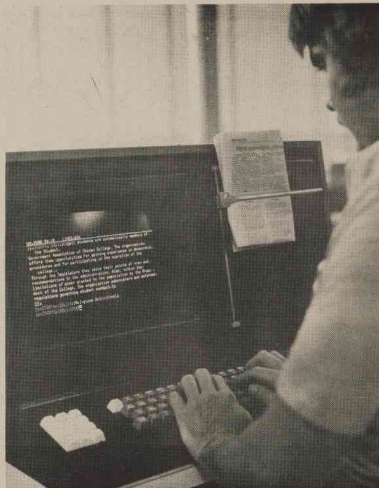
The School of Graphic Communications uses some of the most modern equipment available in its educational program. Student shown is operating a data storage and editing terminal for newspaper typesetting.
