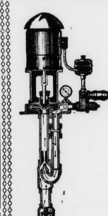
Berkley, the original Hydro-Jet-Deep shallow well pumps. One moving part. Does not have to be installed at well.
