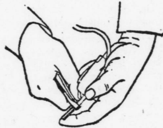
Crimping the Cap to the Fuse.
