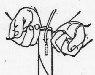
Tying Fuse and Cap to Cartridge.
