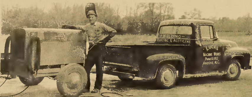
TONY O'MERY of Ahoskie is shown preparing a mobile welding unit for use. The Lucas Company has two similar units that are used for the spot repairs and to allow the shop to work on four welding jobs at the same time. Tony came to Ahoskie from
