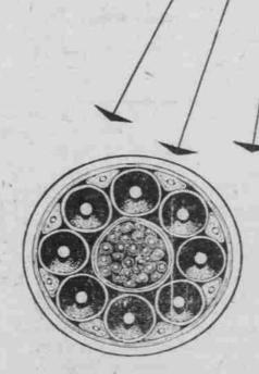
In the old days, it would have taken a pole line over 700 foot high to carry all the conversations that can go through a 21/2-inch coaxial cable
