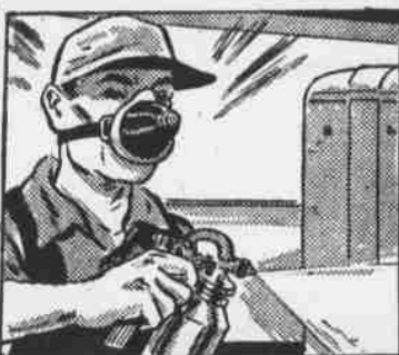
1. Not a gas mask, but a special nose mask to guard his breathing, is worn by this spray painter at his job in one of the General Electric plants.
