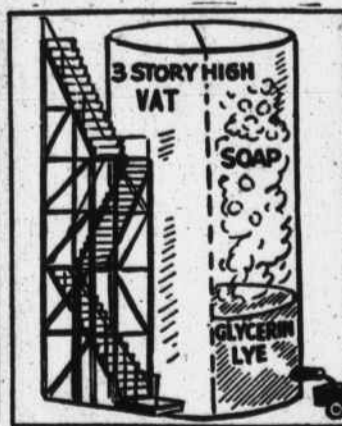
The Tallow is Boiled in Huge Vats, and by Adding Caustic Soda, 88% is Turned into Soap; the Rest Settles to the Bottom as Glycerine Lye.
